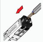
Check there is a sufficient length of outer cable sheath available for clamping.(fig.1) and that an unbroken length of conductor occupies the full extent of the window (fig.2).
