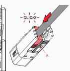
1. After cable termination, close just cover side which includes cord grip (A), then push cable firmly into cord grip (B)
