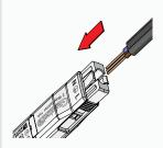
Check there is a sufficient length of outer cable sheath available for clamping.(fig.1) and that an unbroken length of conductor occupies the full extent of the window (fig.2).
