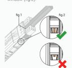
Push cable until it snaps into place. Repeat process for additional cables. Push in any unused cable entries.
