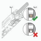
Push cable until it snaps into place. Repeat process for additional cables. Push in any unused cable entries.
