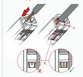
2. Continue to push cable until shuttle snaps into place (A). Repeat process for other outlet or push in unused shuttle
